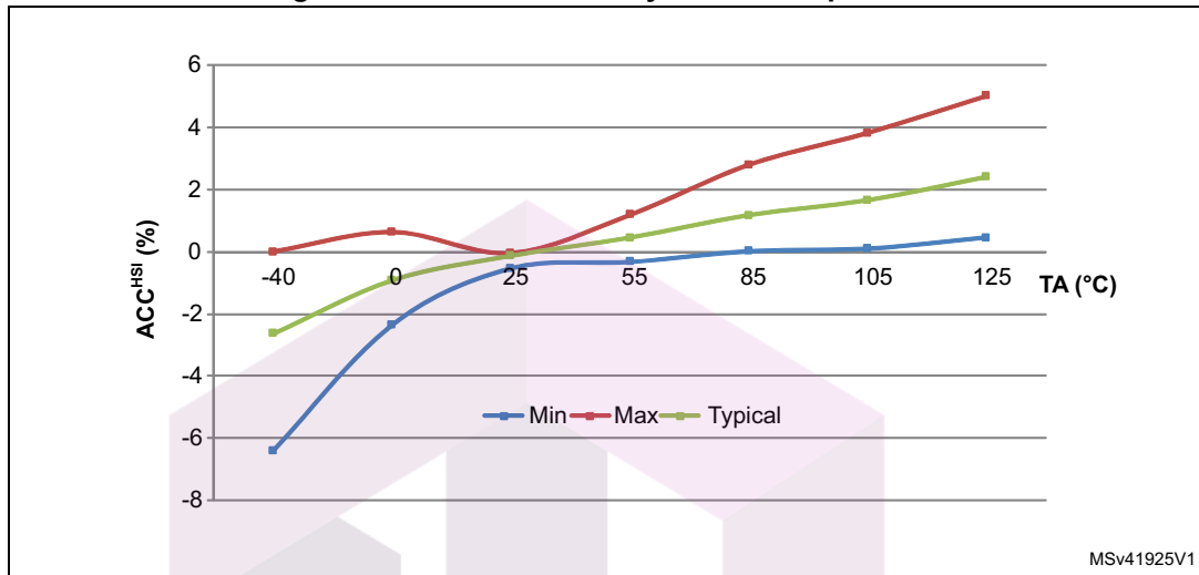
Figure 31. ACCHSI accuracy versus temperature
